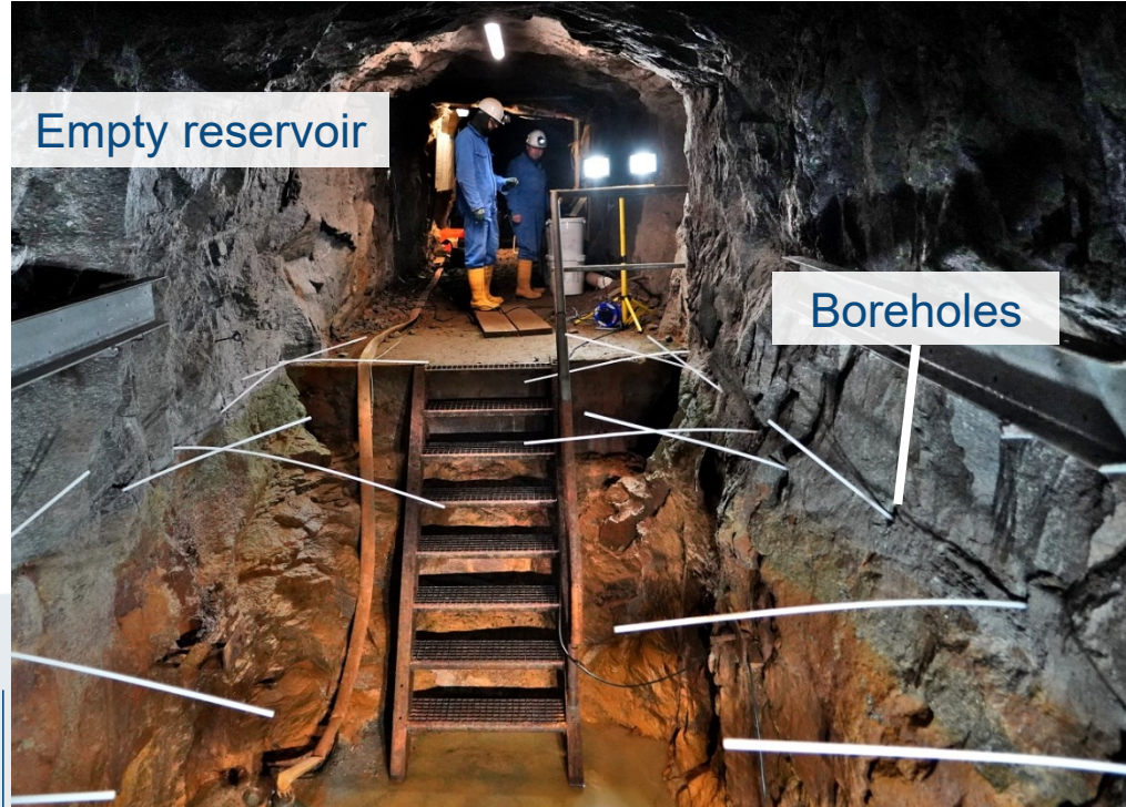
In-situ basin in the Reiche Zeche silver mine with 3 m plastic rods and sensors connected to them
