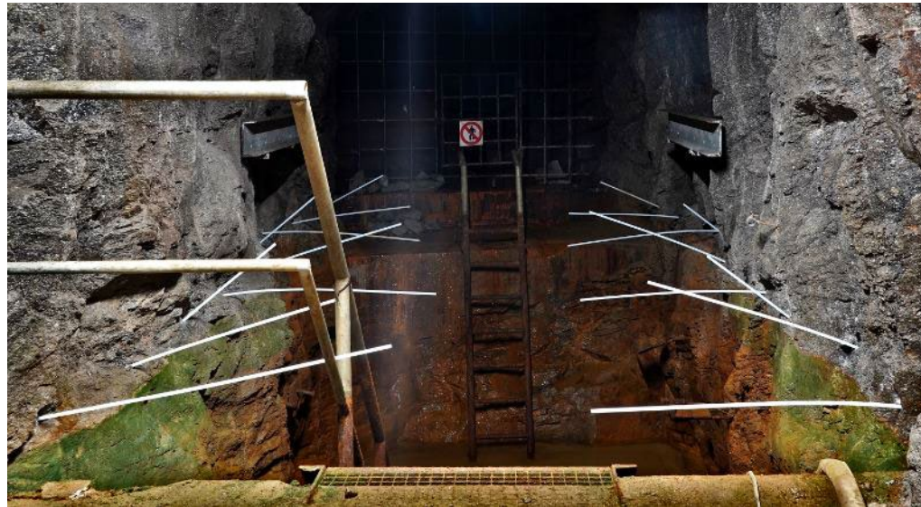
In-situ basin in the Reiche Zeche silver mine with 3 m plastic rods and sensors connected to them
